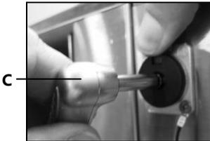
Release the red detent **B**. To remove the probe press the detent **B** again, pull the core temperature sensor **C** and release the detent **B**.
