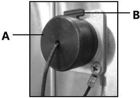
To connect the core temperature sensor take out the plug **A** (image on the left) from the opening at the top left side of the oven, press and hold the red detent **B** and insert the core temperature sensor **C** into the opening provided.
