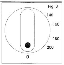
When the green light comes on the appliance is ready to use. The orange light remains on whilst the heating elements are operating
