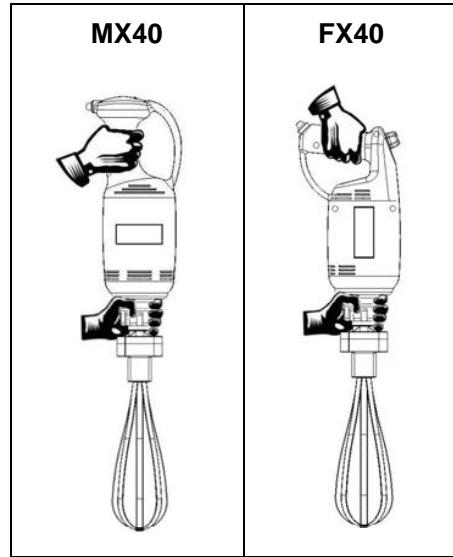
**DANGER – WARNING:** Never near upper limbs or other parts of the body to the area where the mixer utensil is located when inserted in the motor unit. Only clean utensils removed from the motor unit.
