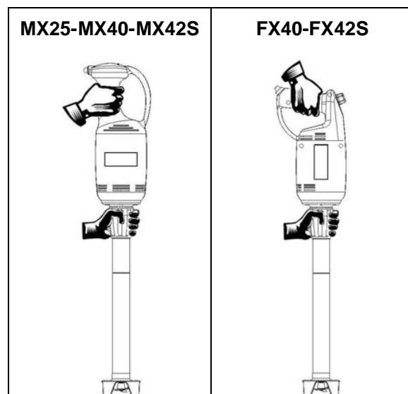
**DANGER – WARNING:** Never near upper limbs or other parts of the body to the area where the mixer utensil blade is located when inserted in the motor unit. Only clean utensils removed from the motor unit.
