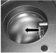
4. Pull the pump tube from the holder and remove it from the can.
