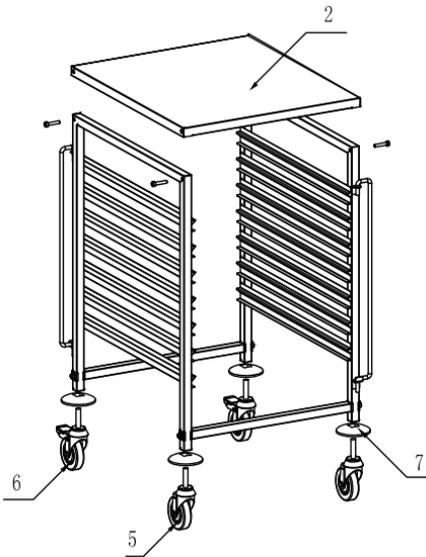
4. Fix the upper storage shelf (2) to the side elements with the use of the supplied bolts.
