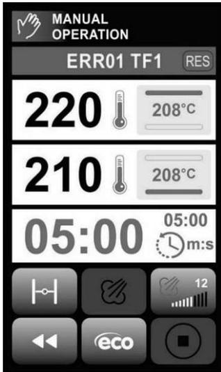
Fig. 30: Manual mode with error display
