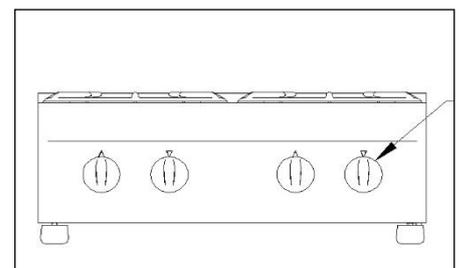
In order to put out the main burner, the knob has to be turned to the right into the on ★ position; as for putting out also the pilot, turn the knob again into the off position ●
