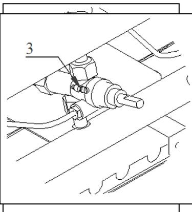
In order to replace the by-pass, it is necessary to remove the knobs (1) and the control panel (2). Then, unscrew the by-pass (3) with a screwdriver and replace it with the by-pass suitable for the gas type to be used, as shown in tables BURNER FEATURES. Reassemble the by-pass and tighten it well. Finally, place back the control panel and the knobs.
