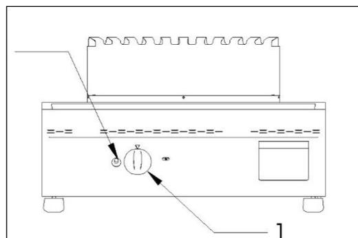
In order to put out the main burner, the knob has to be turned to the right into the position ★; as for putting out also the pilot, turn the knob again, into the off position ●
