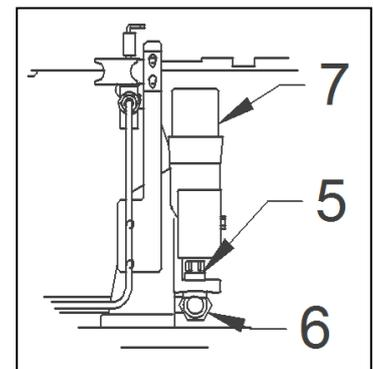
is to be found under the Venturi tube (7) with a spanner and replace it with the nozzle suitable for the
