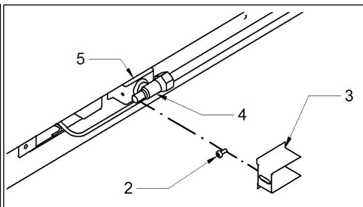
Replacing the burner nozzle
