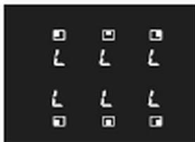
After a few minutes the symbols will disappear. When any dial knob is rotated, however, the above lock symbols will reappear on all displays and the hobs will not activate.
