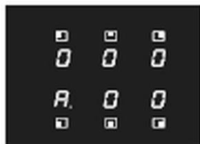
1. Rotate the dial knob counter-clockwise, starting with '0', until an acoustic signal is heard.
