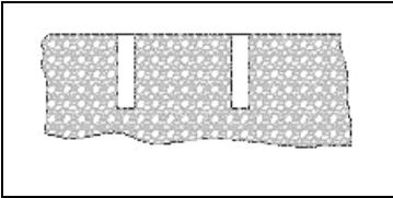
3. Mark the holes in the base plate on the selected position. Then drill 2 holes with a 10 mm stone drill.
