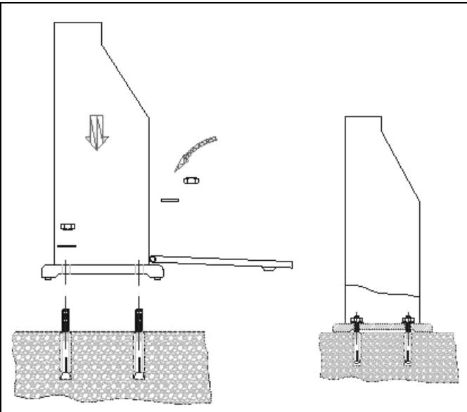
5. Put on the washers and place the free-standing ashtray precisely on the attachments screws of the metal dowels. Then attach the floor ashtray with the nuts and the spring washers.
