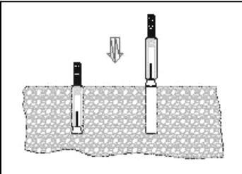
4. Stick the metal dowels with the attachment screws into the drilled holes in the ground as illustrated.
