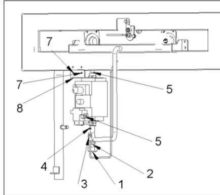
In order to replace the safety valve, remove the water and gas knobs and the crank; then remove the front panel by unscrewing the four screws that hold it in its place. Unscrew consecutively the pipe union that leads to the
