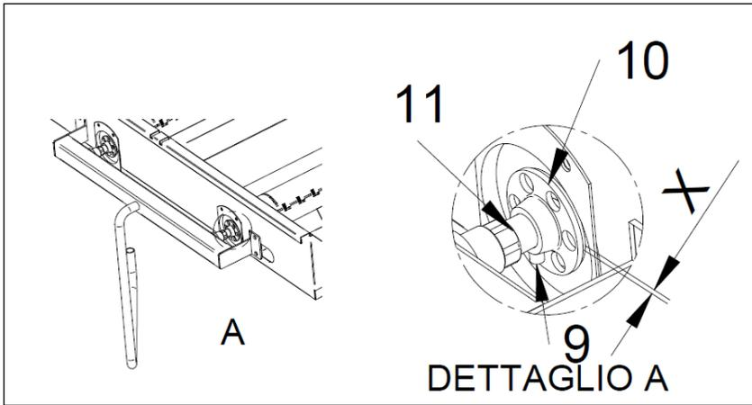
In order to replace the burner nozzle, remove the knobs (1) and the lifting crank (2); then remove the front panel (3) by unscrewing the 4 screws that hold it in its place (4). Unscrew the connection (5) that joins the ramp (6) to the electro-valve (7) and the screws (8) that fix the electro-valve to the appliance frame. After clearing the work area, loosen the screw (9) that blocks the primary air
